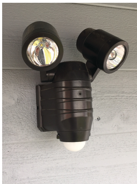
Figure 2. Automated light that is reactive to motion in the dark. Configuration allows the setting of thresholds for sensors and timings. Interventions prolong or terminate the light exceptionally.
