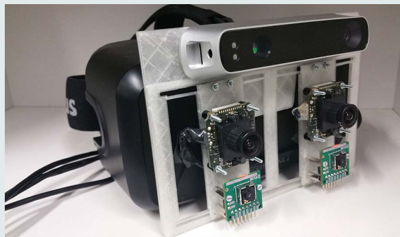
Figure B. Feuerwerr project. To the front of the display, two RGB cameras, two thermal cameras, and a depth camera are attached. In the face mask, physiological sensors are built-in to allow intuitive user control.
