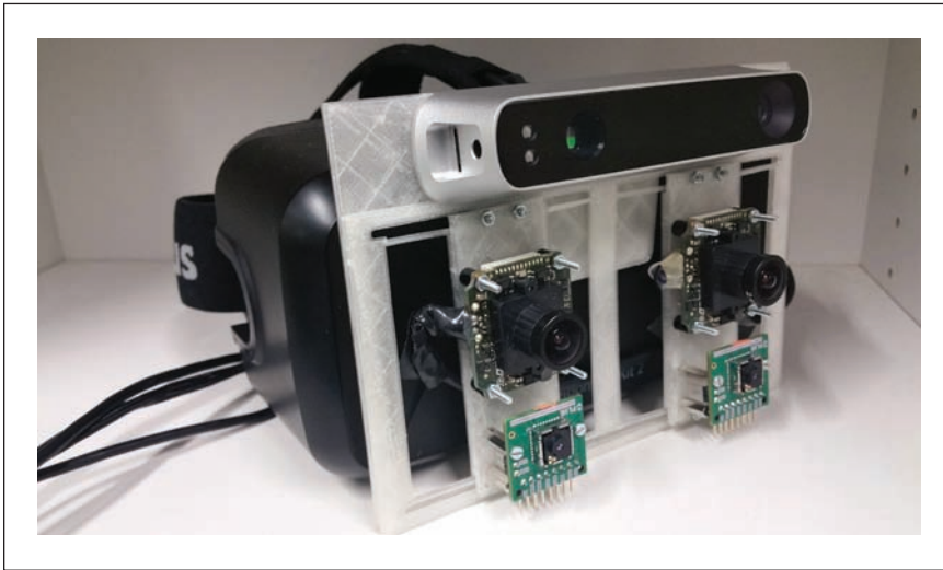
Figure 1. Prototype of a video see-through system that combines an Oculus with an RGB, depth, and thermal image and allows implicit control by different physiological sensors. (Source: Yomna Abdelrahman and Pascal Knierim, Project FeuerWeRR, University of Stuttgart; used with permission.)
